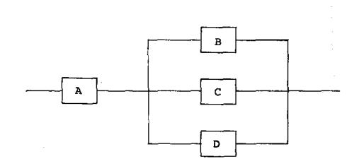
In the above system, a system failure consists of a failure of either component A, or a failure of at least two of B, C, D.
